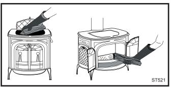
**Fig. 22** Top loading is the best way to add fuel during regular use. Front loading is useful for kindling a fire.
